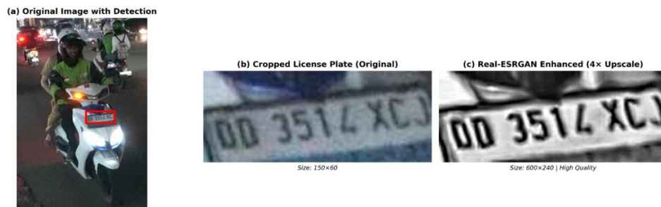
Figure 2. Image enhancement comparison using Real-ESRGAN under low-light conditions
